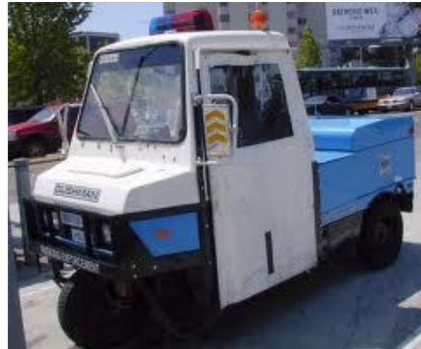
The function slowly improved by adding sliding doors. The overall compact size is always key to minimize traffic interruption
