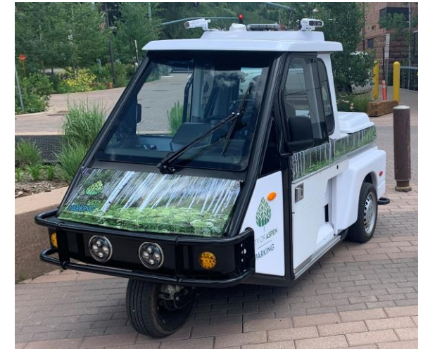
Newer versions allow traditional chalking or installation of technologies, EVs also available reducing carbon footprint. Safety has been improved dramatically with roll bar chassis. Ease of use with automatic transmissions
