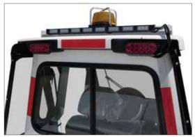
LED lighting is now a standard feature in the GO-4, for all exterior lighting other than the head lights. Lighting is also positioned up high on the rear cab to easily notify vehicles of frequent stopping. Additional beacons can be added.
