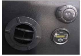
Optional AC is available, as well as a lateral thrust alarm which notifies the driver if taking a corner too quick and tight.
