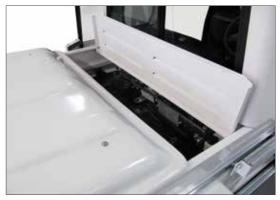
Rear engine lid provides easy access for checking oil and coolant levels
