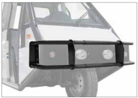
Additional nerf bar option for reducing impact from any potential dents and collisions.
