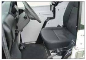
A comfortable interior offers an adjustable sliding chair, tilt steering, excellent viewing conditions, and optional cup holder arm rest.
